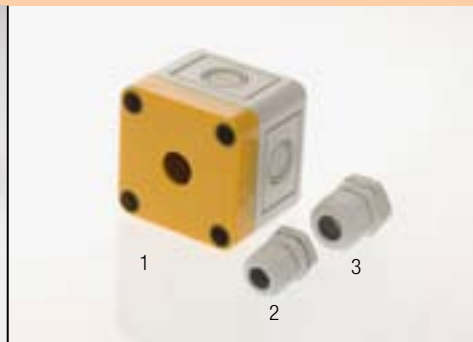
Emergency-stop switch enclosure with 22.5 mm Ø mounting hole, 65 mm (w) x 65 mm (h) x 57 mm (d), anti twist hole. Cable gland M16 or M20, IP66
