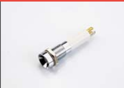
Indicator, internal reflector, 5 mm LED, 24VDC, 8 mm mounting, bi-colour
