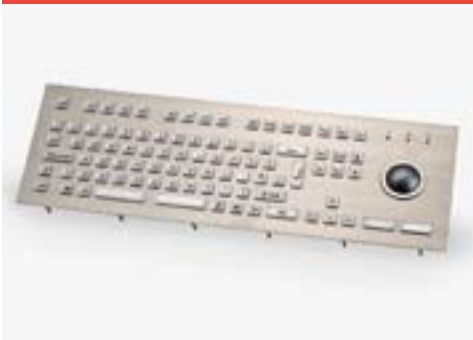
Alphanumeric keyboard, top mounting, 91 keys, optical trackball, 6 rows/MF2, 2 clicks, PS2 and USB output types, English, German, French and US English layouts
