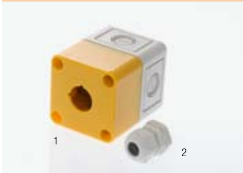
Emergency-stop switch enclosure with 22.5 mm Ø mounting hole, 65 mm (w) x 65 mm (h) x 81 mm (d), anti twist hole. Cable gland M20, IP66
